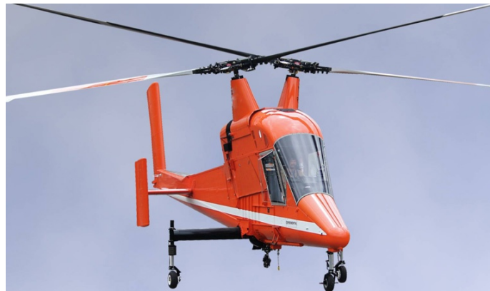
Image 9 Kaman K-Max 6,000 lbs lift capable
