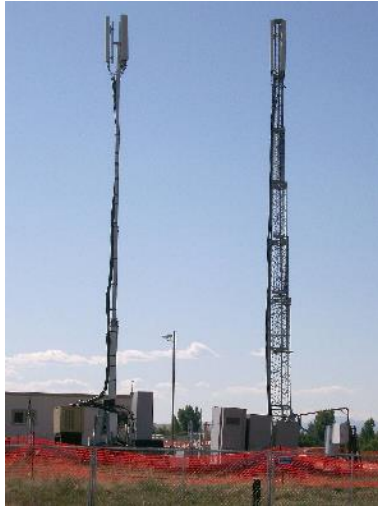
Image 6 A deployed cell on wheels (COW)
