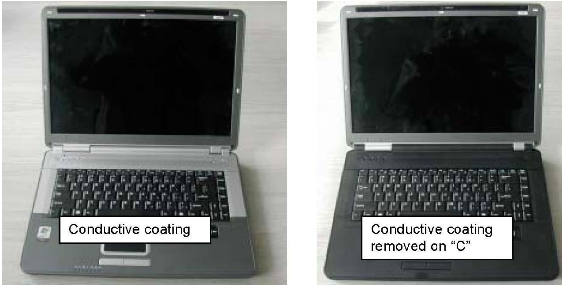
Figure A.3 – Installation of a “C” Shell (with and without conductive coating on the top side) on complete system
