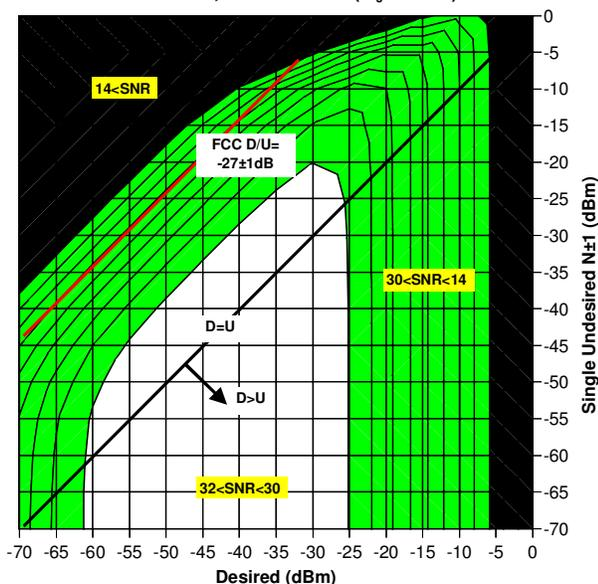
Figure 1b: Receiver Post-decoder SNR Conours (2dB interval)
