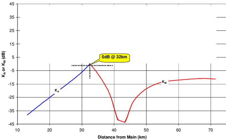
$K_A$  and  $K_M$ , shown in Figure A5, are functions of the Main-Aux separation distance. The distance to crossover point,  $K_A = K_M = 0\text{dB}$ , is controlled by the radiation patterns, the antennas' height and the ERP of each station. If the Auxiliary uses a directional antenna, the crossover point will move further toward the RH of the Main. The receiver's switches between the Main and Auxiliary channels depending on the higher SNR of these two desired channels.
