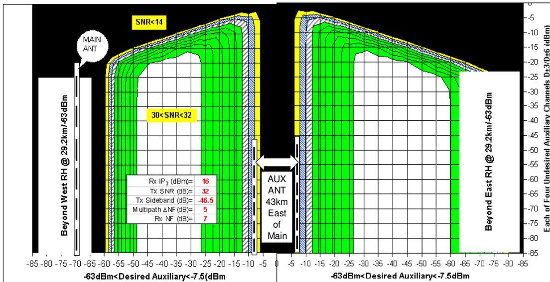
Figure 6: Post-decoder SNR Contours (2dB intervals) of Auxiliary-22
