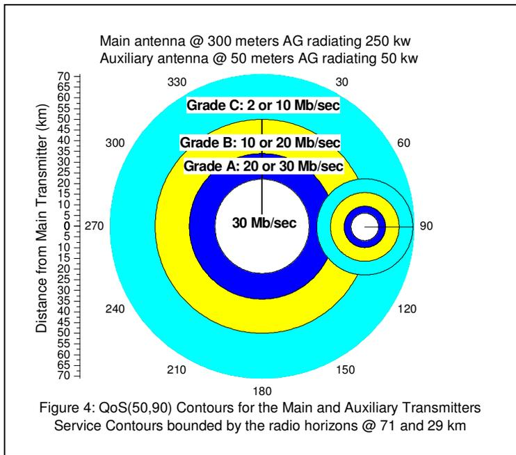
Figure 4: QoS(50,90) Contours for the Main and Auxiliary Transmitters Service Contours bounded by the radio horizons @ 71 and 29 km
