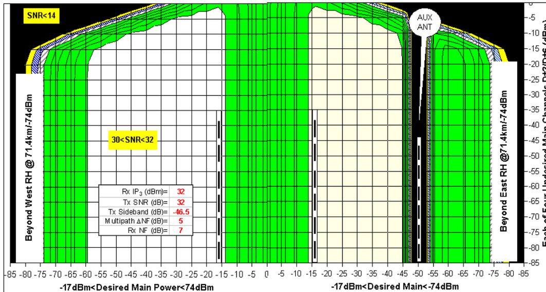
Figure 7: Post-decoder SNR Contours (2dB intervals) of Main-23
