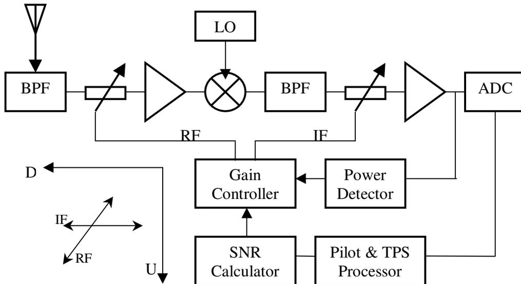
Figure 2: Modified AGC for Adjacent Channel Reception Optimization
