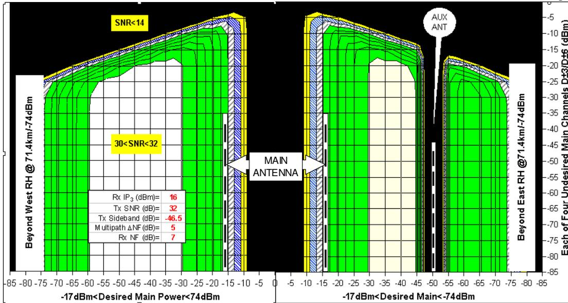
Figure 5: Post-decoder SNR Contours (2dB intervals) of Main-23
