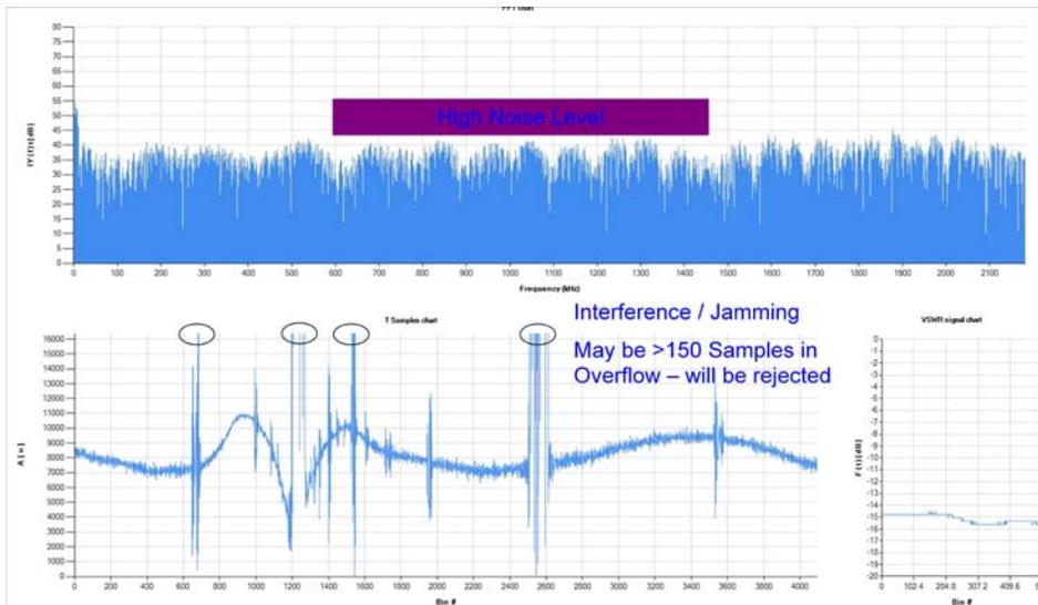
The following example demonstrates the effect of multiple jammers crossing the swept signal bandwidth and then creating multiple intermodulation effects. The noise floor has been completely destroyed and the number of A/D samples that are in saturation as the receiver is also saturated approaches a large fraction of the total data collection period. This data is unusable and if not detected and eliminated by the altimeter will cause serious operational problems.
